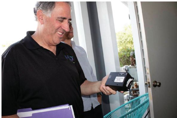
Don Millstein, H2O Degree President, shows the MachineQ team the LoRa 2-Channel Pulse Counter.
