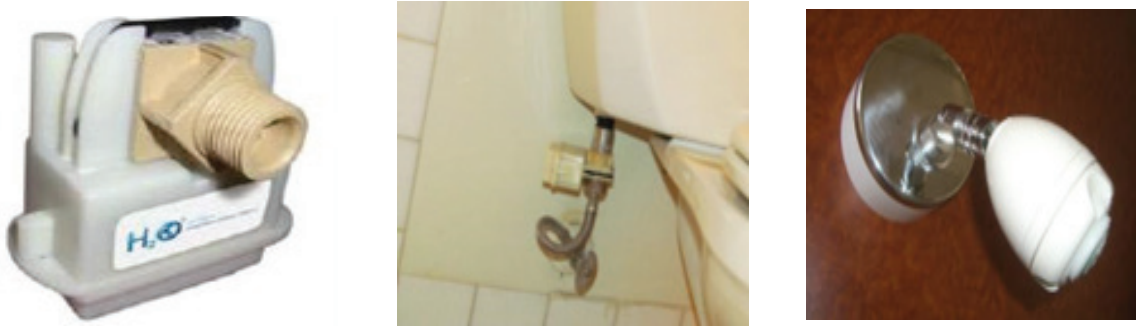
Figure 2. Battery-powered wireless water meters measure water consumption at point-of-use entry locations like toilets and showers. The meters can track granular data to evaluate “events” (flushes, etc.) for each toilet in a multi-unit apartment to detect leaks.
