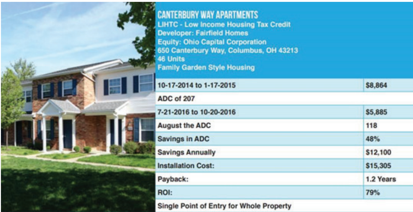
Figure 4. LIHTC property realized payback on the installation of wireless submetering after only 1.2 years.
